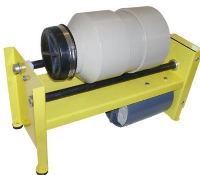
Figure 22: Ball mill representation
