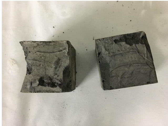
Figure 52: Broken specimens of CB with SEBS showing much less damage at failure
